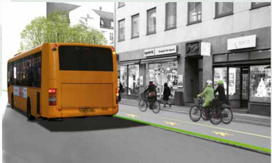
▲Dynamic bus stops use remotely controlled dynamic markings to create virtual traffic islands which vary the width of the cycle lane allowing space for passengers to get off buses and then returning the lane to the full width ▼
