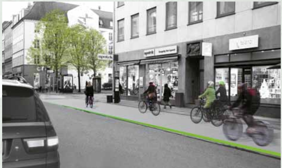
▲Dynamic bus stops use remotely controlled dynamic markings to create virtual traffic islands which vary the width of the cycle lane allowing space for passengers to get off buses and then returning the lane to the full width ▼
